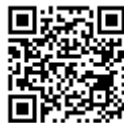
Figure 8. A QR code of base 64 encoding of the document number 1 and SHA-256 of the title of this paper.
